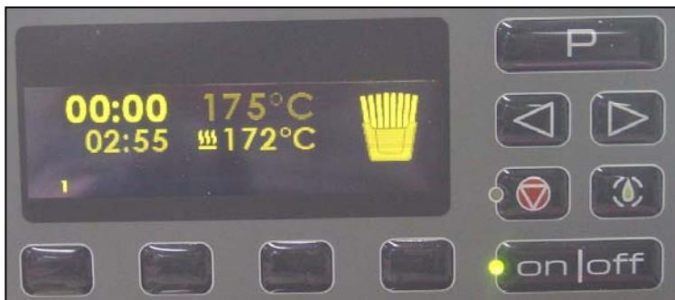
The count down indication flashes „0.00“ and an acoustic signal informs the operator.
