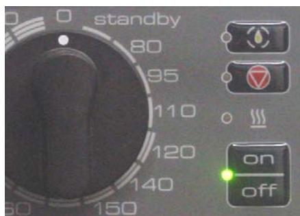
Press the "ON" Button to put the control panel under tension.
