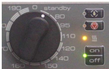
The „Standby“ position is also the fat melting cycle (FMC). This position allows to heat up slowly to 60°C. The heating element switch on and off during this cycle in order to melt fat and to heat up fat and oil without smoke and increase the lifetime of the fat and oil.
