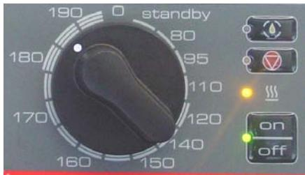
By turning the knob clock wise you can select the requested frying temperature.
